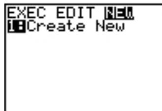
2. Press **[ENTER]** to select **1: Create New**. The **Name=** prompt is displayed, and alpha-lock is on. Type in **[A][S][E][C][T][O][R][D]** as the name of your program.
